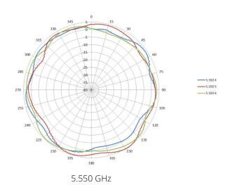
Elevation plane (side view, 0 degrees angle)
